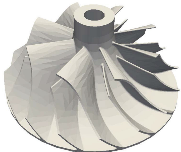
Fig. 1. Centrifugal impeller STL file domain used for the thermal simulation at the component scale. Open source STL file is obtained from [28]. The diameter of the impeller is d = 65 mm and the height of the impeller is h = 31 mm.
