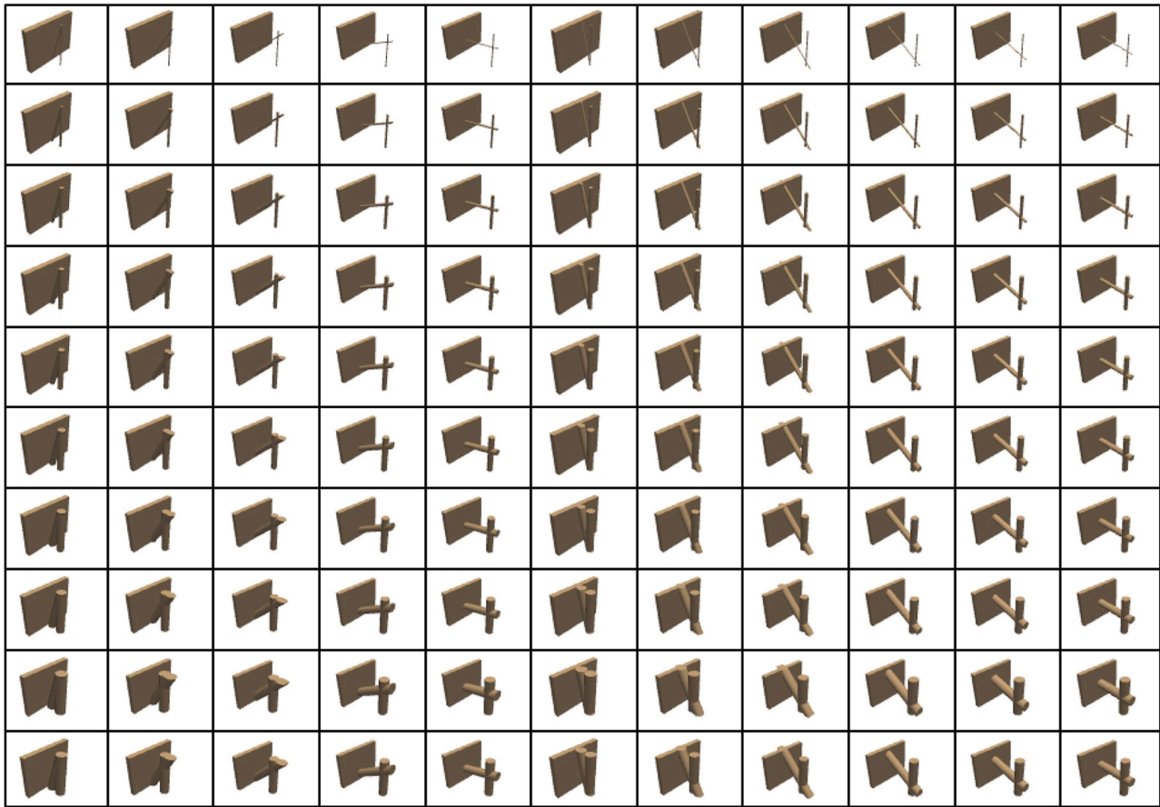
Fig. 1. All the circular strut features designed by FreeCAD and Python script.
